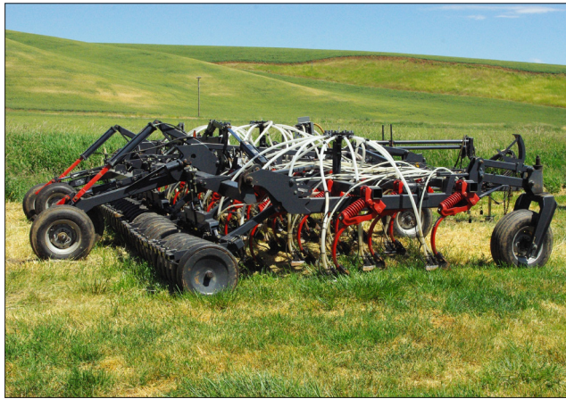
Figure 17. After trying several different drills for oilseeds, Clay modified a direct-seed shank drill in 2011 to plant mustard and canola.
