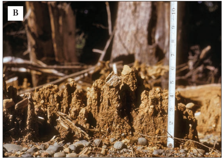
Figure 19. Unless guided into the forest to be filtered, erosion from forest roads can degrade adjoining stream water quality (A) and create small castle-like columns under gravel and rock. A 6-inch erosion depth suggests that as much as 50 cubic feet of soil could have been lost from a 100-square-foot area (B).
