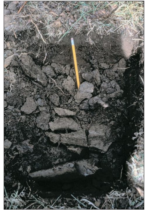
Figure 13. Platy structure in a silt loam soil indicates soil compaction. This was caused by repeated equipment traffic during timber harvest eight years earlier under wet conditions. Such soils have lost nearly all structure and productivity.
