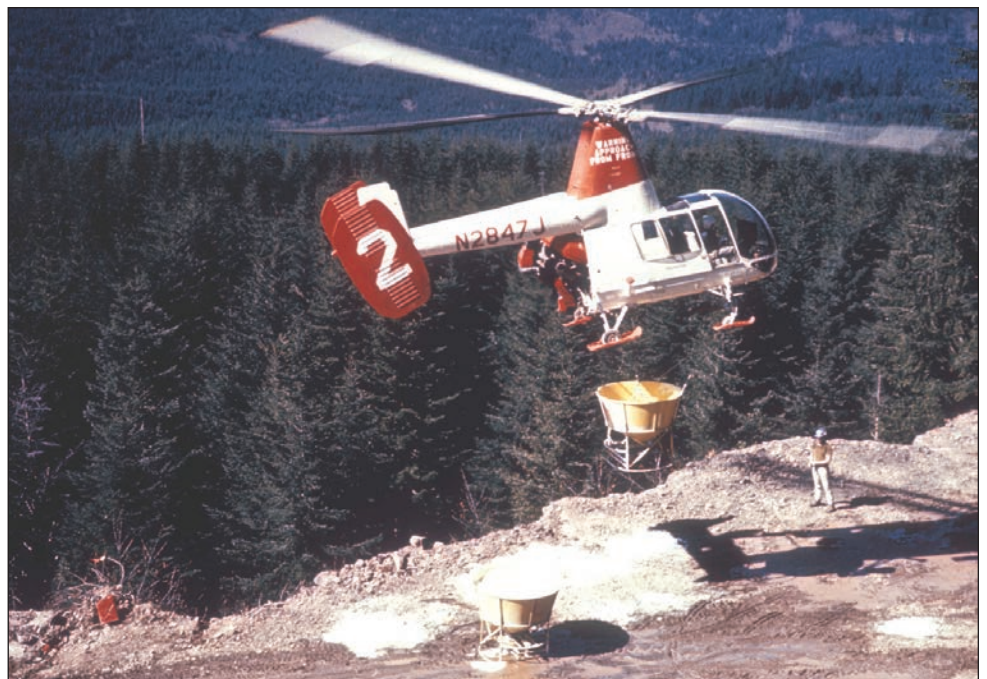
Figure 17. Helicopters are the usual means for spreading fertilizer in Northwest forests. For smaller projects, tractor-mounted or even human-carried centrifugal spreaders work well.
