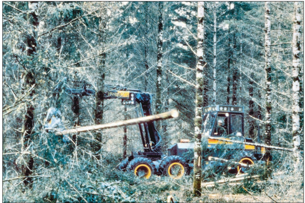
Figure 14. Cut-to-length harvesters can place a mat of branches ahead of the machine to protect forest soil.
