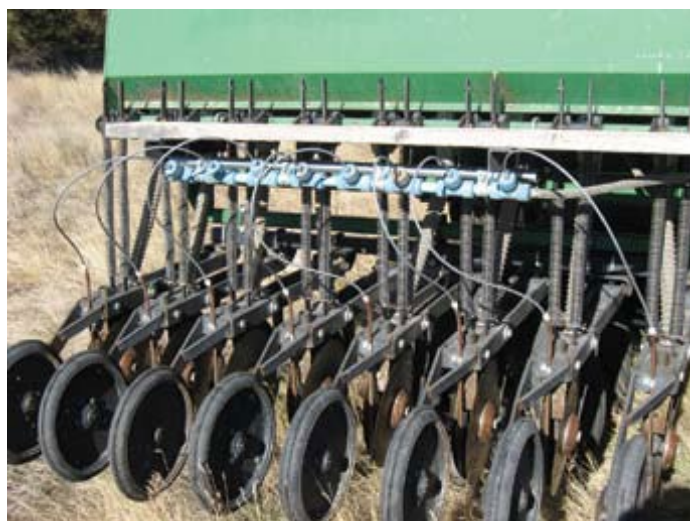
Figure 7. Disc drill modified to place liquid starter fertilizer in the seed row.
