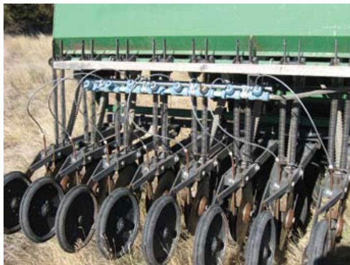
Figure 9a. Disc drill modified to place liquid starter fertilizer in the seed row.
