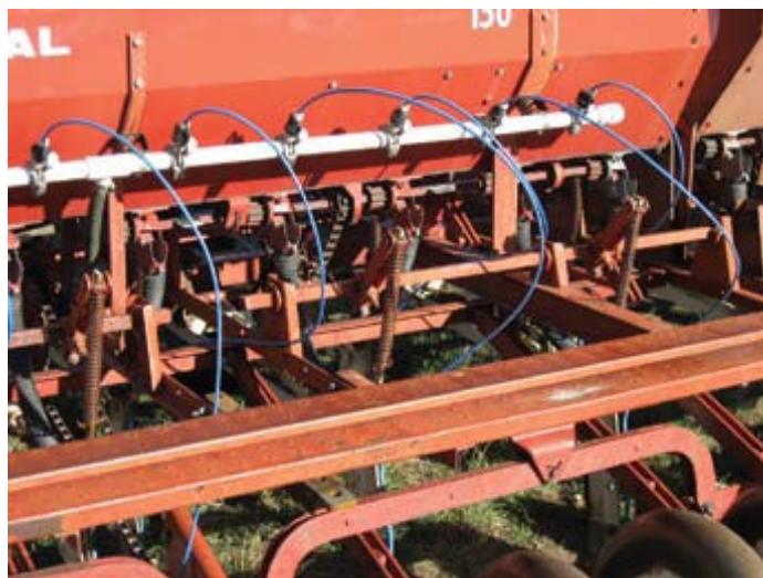
Figure 9b. Hoe drill modified to place liquid starter fertilizer in the seed row.
