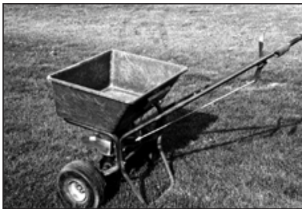
Typical broadcast fertilizer spreader for pelleted fertilizer.
