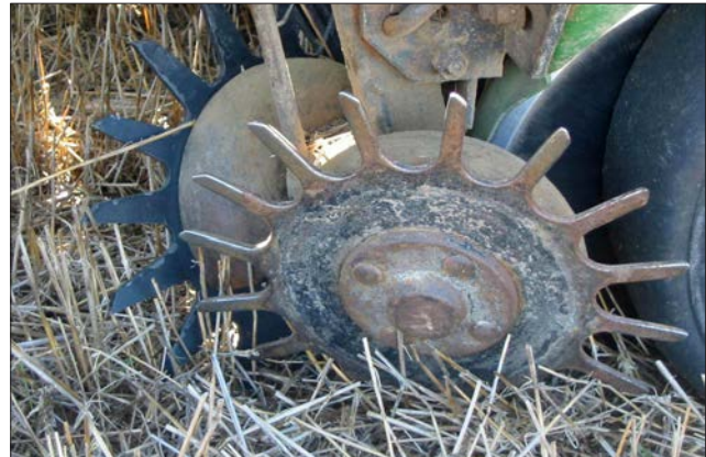
Figure 16. Row cleaners move residue off the planted row.
