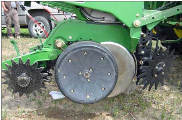
Figure 28. Planter-row-unit retrofitted for direct seeding.
