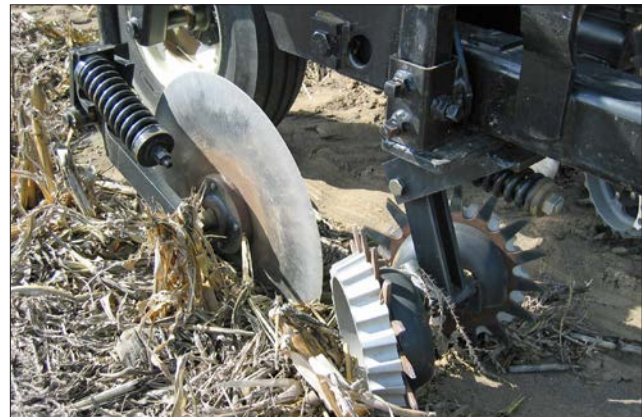
Figure 17. Floating row cleaners preceded by a smooth coulters. These maintain their height, "floating" over uneven ground.
