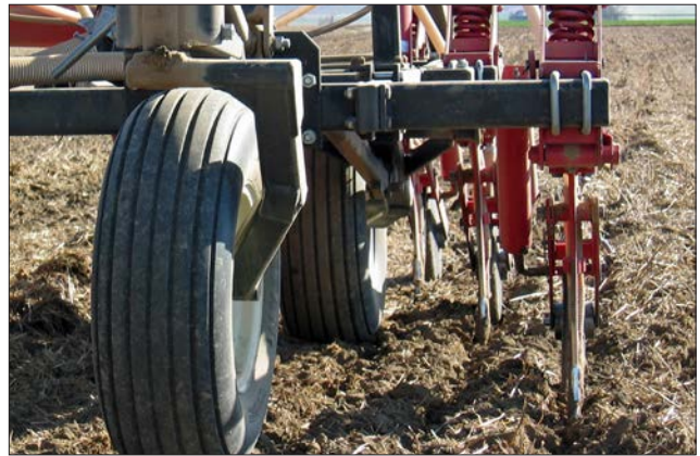
Figure 29. Drill openers mounted on different ranks to facilitate the flow of residue between openers.
