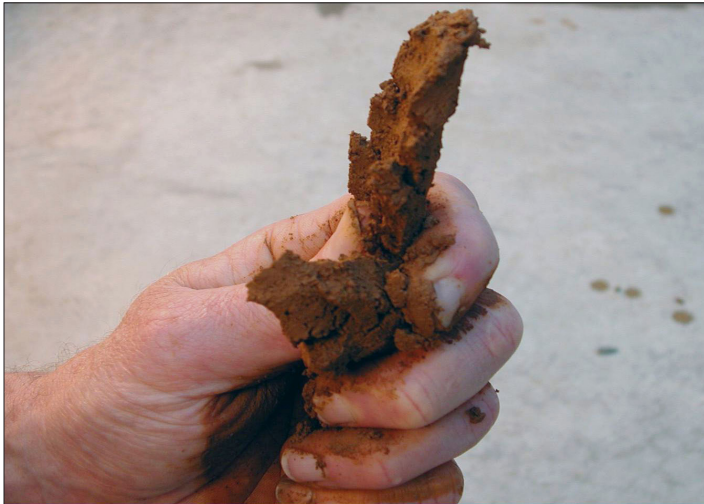
Figure 2. Determining soil texture by feel. For example, the pictured soil sample holds its shape after being pressed, indicating a high clay content. Photo by Andy Bary.
