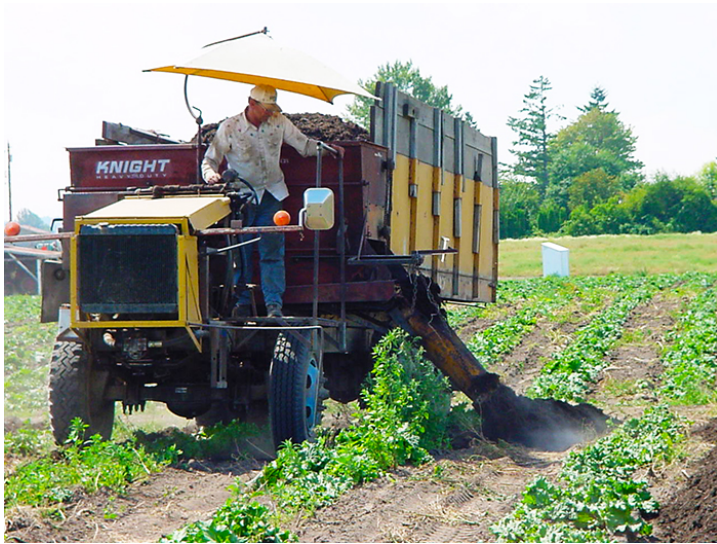
Fig. 2. Applying yard trimmings to rhubarb using a spreader adapted for delivery between rows.
