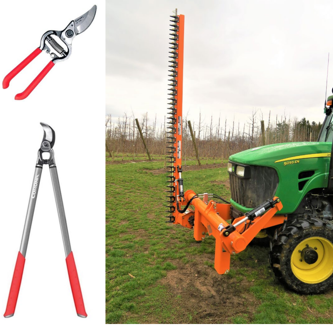
Figure 1. Hand-held pruner (top left), lopper (bottom left), and tractor-mounted hedger (right). (Images by T.R. Alexander, WSU; Dan LaGasse, LaGasse Works.)
