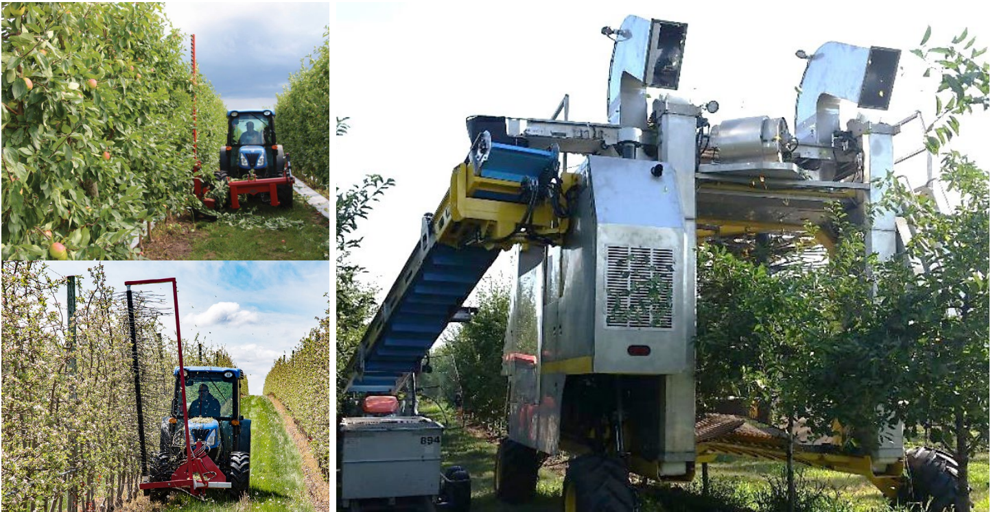
Figure 3. Mechanized thinning (top left) and pruning (bottom left) of apples, and mechanized harvesting of tart cherries (right). (Photos by R.J. Anderson, Cornell Cooperative Extension; Christina Herrick, Western Fruit Grower; Dan Setniker, Littau Harvester.)
