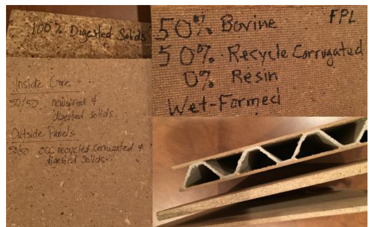
Figure 9. Particleboard samples made from AD fiber. (Photo courtesy of DVO Inc.)
