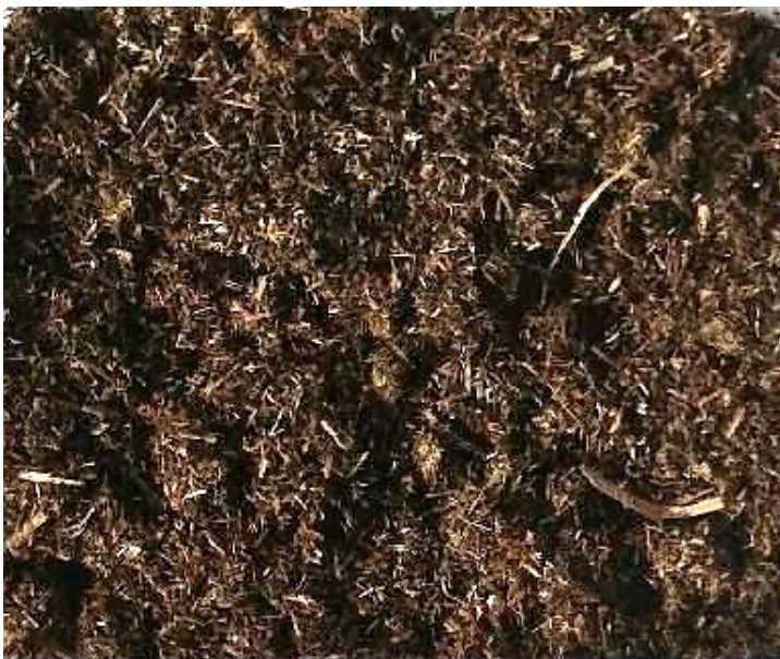
Figure 2. Screened and pressed fibrous solid from AD effluent. (Photo courtesy of Craig Frear.)
