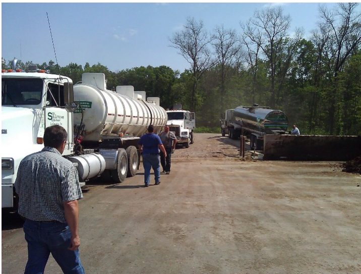
Figure 7. Trucks hauling substrates to receiving pits should be provided enough space to avoid congestion between haulers. (Photo courtesy of DVO, Inc.)
