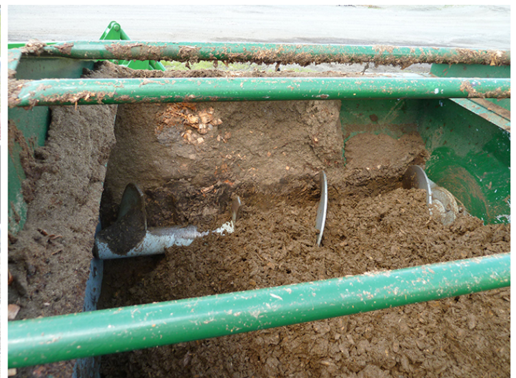
Figure 3. Mechanical mixers installed in this receiving pit homogenize the slurry (left), while an auger mixes food wastes with dairy manure (right). (Photos courtesy of Jim Jensen and WSU Energy Program.)
