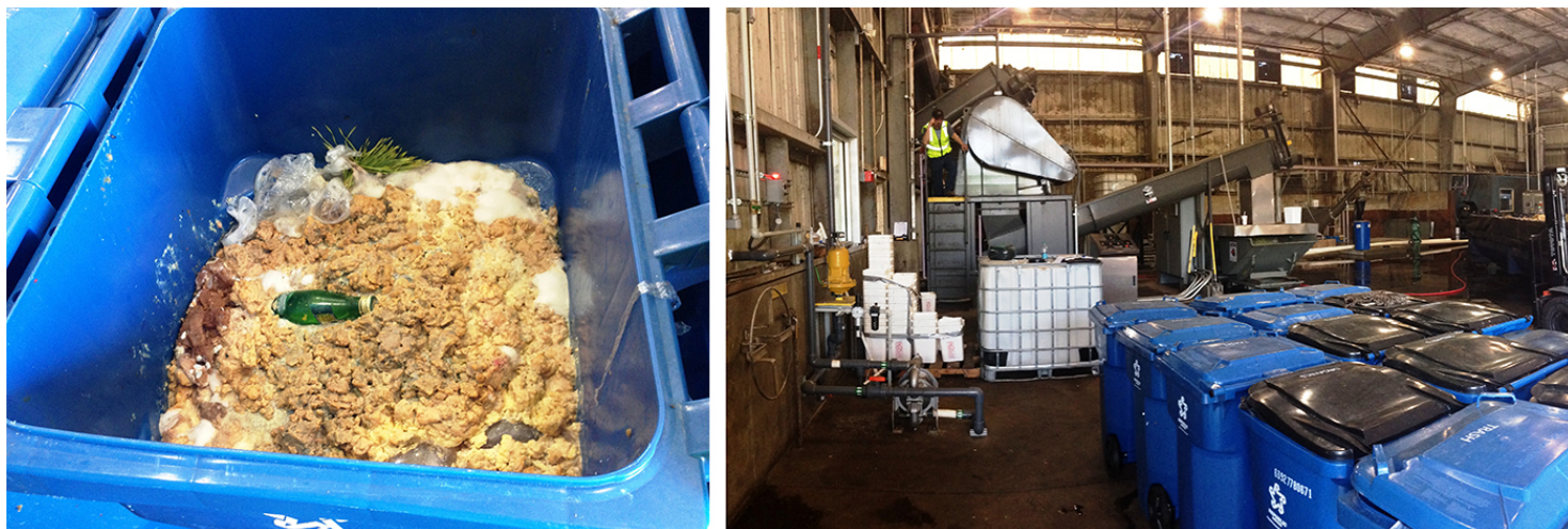
Figure 2. Substrates can contain unwanted material such as plastics and bottles (left); prescreening facilities (right) use separation equipment to remove inorganics from organics prior to AD. (Photos courtesy of American Biogas Council.)
