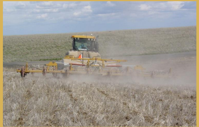
Figure 3. An undercutter implement minimizes soil lifting and allows most of the residue to remain on the surface. Blowing dust emissions are reduced by 70 percent with undercutter tillage compared to conventional tillage methods. The tank cart in front of the undercutter contains aqua ammonia nitrogen and thiosol sulfur that is injected through tubes running on both sides of each V blade on the undercutter. Photo: Bill Schillinger.
