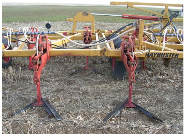
Figure 1. The undercutter has overlapping 32-inch-wide narrow-pitch V blades on two tiers to slice below the soil surface at a depth of five inches, completely severing soil capillary pores and channels. This retains seed-zone moisture during the hot, dry summer months. Photo: Bill Schillinger.
