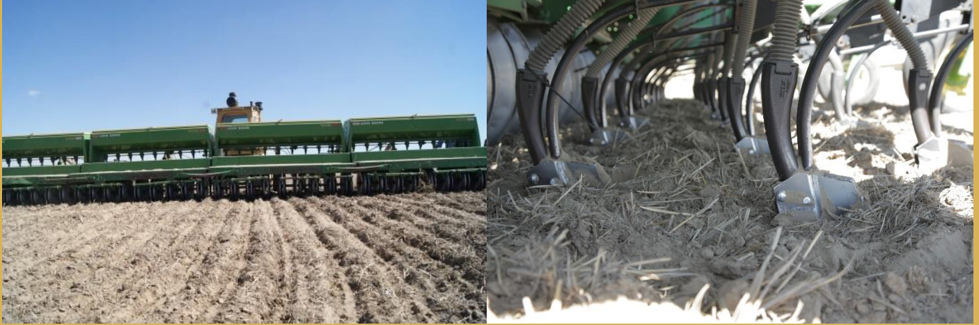
Figure 10. Jirava’s John Deere 9400 drill (left), with close-up of shanks (right). Among the features that allow it to penetrate heavier residue well are the heavier shank and leaf spring assembly along with the staggered seed openers. Photos: Hilary Davis (left) and Darrell Kilgore (right).
