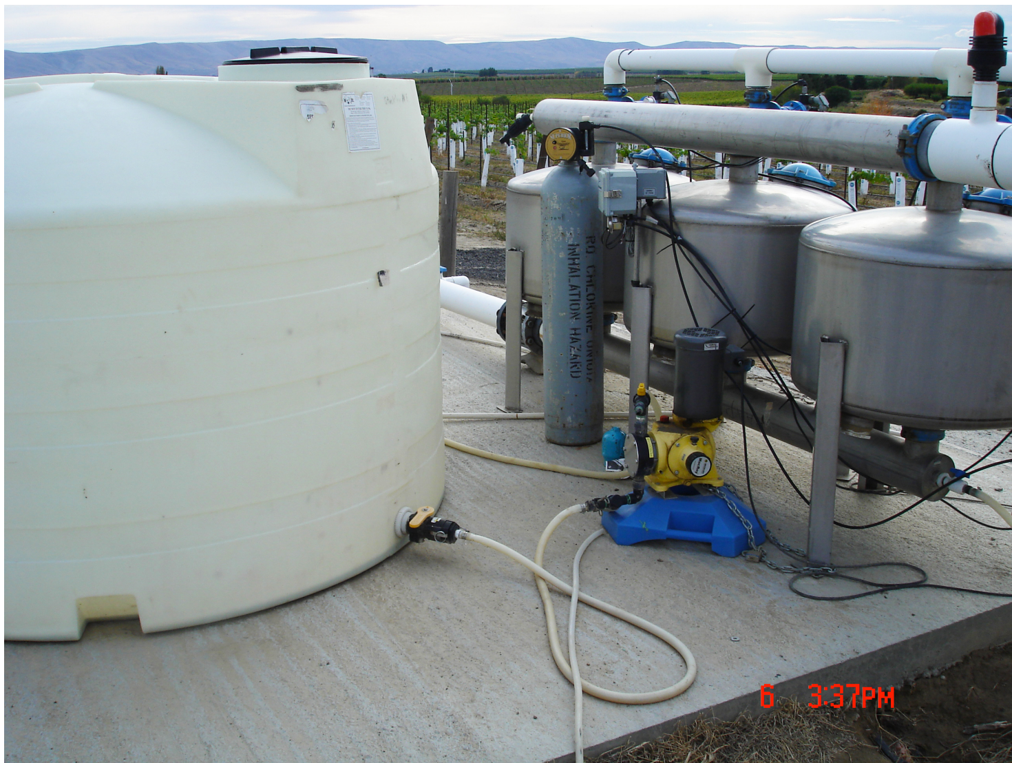
Chemigation pump set up to inject fertilizers and agricultural chemicals for distribution to field crops with the irrigation water.
