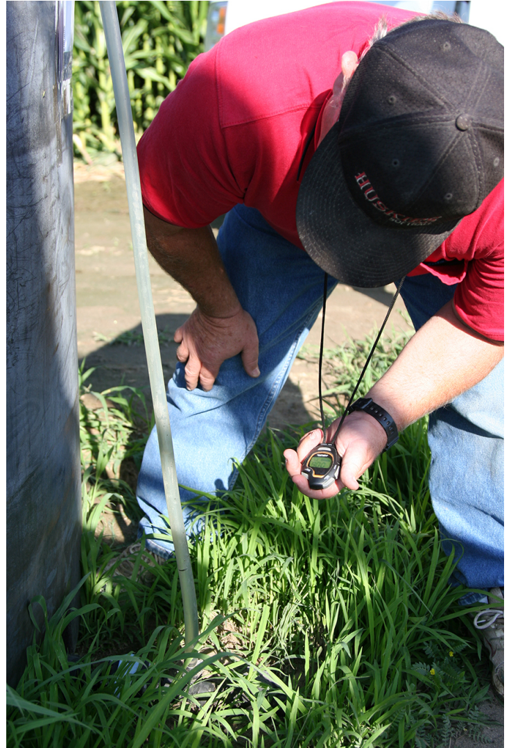
Figure 2. Applicator is measuring the distance that the fluid level changed in the external site tube during the calibration time period.
