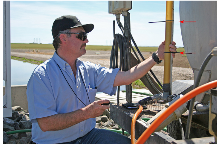
Figure 3. Notice bands that are used to delineate fluid level in calibration tube at the start and then at the end of the calibration timeframe.
