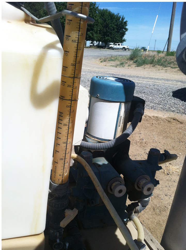
Figure 6. A graduated calibration check tube.
