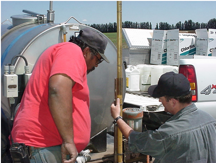
Figure 1. Performing a chemigation injection pump calibration.
