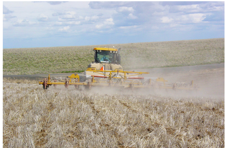
Figure 2. An undercutter implement with V-shaped blades being used for primary spring tillage plus fertilizer injection during the spring of the fallow year. Scientists and farmers have conclusively shown that use of the undercutter implement for primary spring tillage effectively retains equal seed-zone and total profile soil water and significantly greater surface residue compared to TTF implements, such as a tandem disk or field cultivator. Photo by W.F. Schillinger, WSU.
