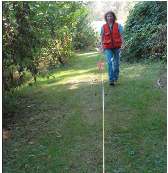
Figure 3-1: Mark out a distance of 1 chain (66 feet) in a flat area such as your lawn or driveway. Walk this distance several times, counting your paces as you go.
