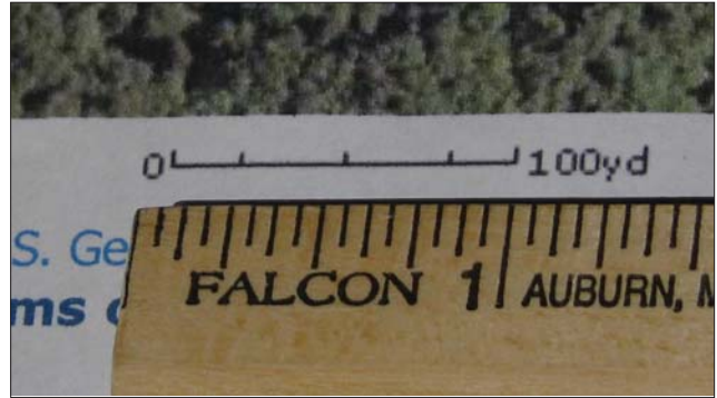
Figure 2-1: The scale of this aerial photo is approximately 15/16ths inches = 100 yards (300 feet).
