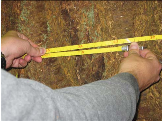
Figure 6-1: To measure DBH, wrap a diameter tape around the tree at breast height, making sure the tape is level and not twisted. Read the diameter measurement where the tape overlaps with the zero marker. In this case, the DBH of this tree is 34.0 inches.
