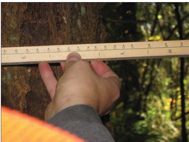
Figure 6-2: To measure DBH with a woodland stick, hold the stick against the tree at breast height, 25 inches from your eye. Keeping the stick level and perpendicular to your line of sight, line the end up visually with the left side of the tree. Then move your eyes (not your head) to read the diameter on the right side of the tree. In this case, the tree whose DBH measured 34.0 inches with the diameter tape in Figure 6-1 measures between 33 and 34 inches with the woodland stick.
