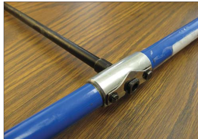
Figure 6-12: An increment borer is assembled by inserting the back end of the bit into a notch in the center of the handle and clipping into place.
