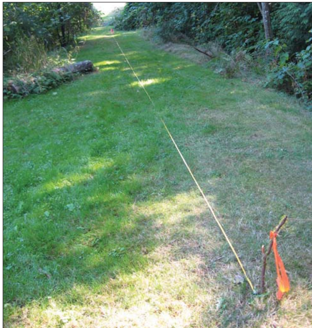
Figure 3-1: Mark out a distance of 1 chain (66 feet) in a flat area such as your lawn or driveway. Walk this distance several times, counting your paces as you go.
