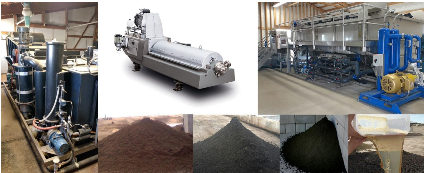
Figure 3. From left to right, top; belt press polymer/flocculation system, decanting centrifuge (photo GEA), DAF polymer/flocculation system. From left to right, bottom; as-produced solids from three respective technologies, and sample of tea water effluent from the DAF (photo DVO, Inc.). Photos: Regenix except as otherwise noted.
