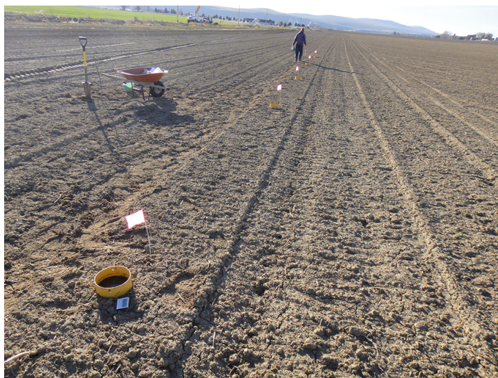
Figure 1. Conducting infiltration measurements along a field transect.
