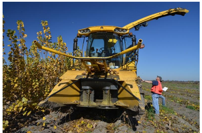
Figure 12. New Holland developed a coppice header for use on a traditional forage harvester. This equipment is used to harvest poplar and willow grown on two-, three-, or four-year rotations.
