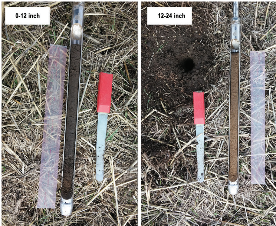
Figure 2-1. A darker color of the surface soil (left) indicates the presence of higher organic matter content compared to the subsoil (right). (Photo by Rakesh Awale.)
