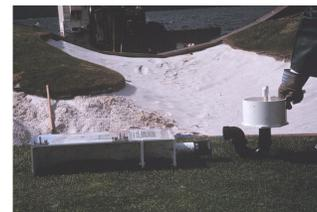
Fig. 2 - Trapezoidal flume assembly
