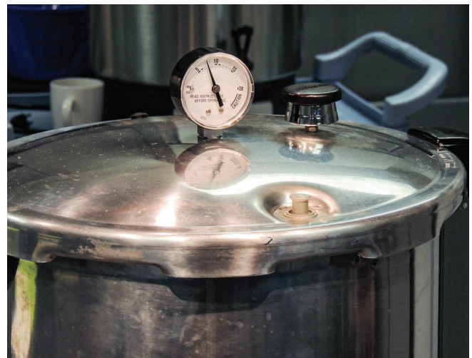
Figure 6. The dial gauge is a delicate instrument and must be tested each year for accuracy. Courtesy of Colorado State University.
