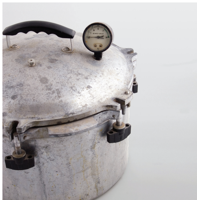
Figure 10. Pressure canner with corrosion and pitting.
