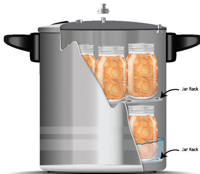
Figure 3. A 23-quart canner allows for stacking pint jars for processing.
