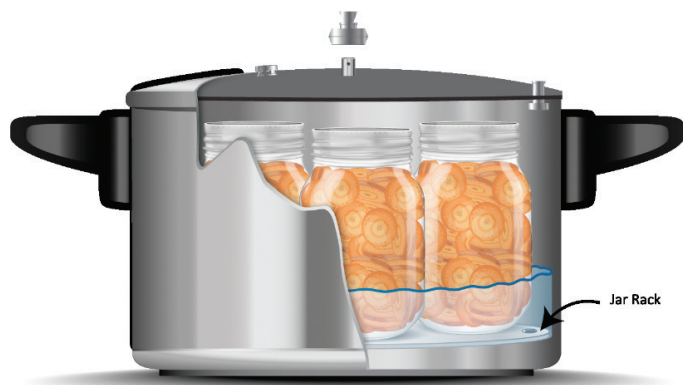
Figure 2. A 16-quart pressure canner allows for processing pint and quart jars in a single layer.
