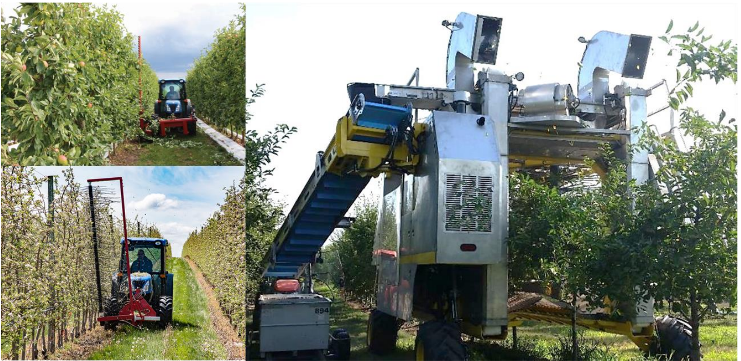
Figure 3. Mechanized thinning (top left) and pruning (bottom left) of apples, and mechanized harvesting of tart cherries (right). (Photos by R.J. Anderson, Cornell Cooperative Extension; Christina Herrick, Western Fruit Grower; Dan Setniker, Littau Harvester.)
