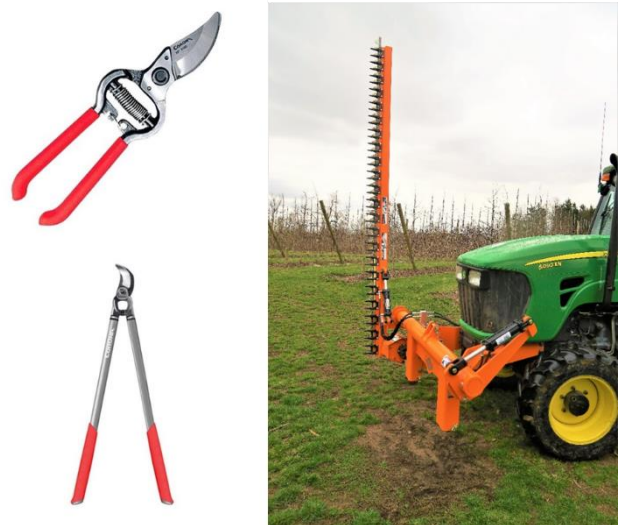
Figure 1. Hand-held pruner (top left), lopper (bottom left), and tractor-mounted hedger (right). (Images by T.R. Alexander, WSU; Dan LaGasse, LaGasse Works.)
