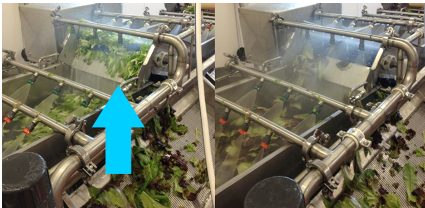
Figure 1. Lettuce cultivar with a flat leaf structure tends to clog processing equipment (left), whereas cultivars with looser leaves pass through the equipment more easily (right).
