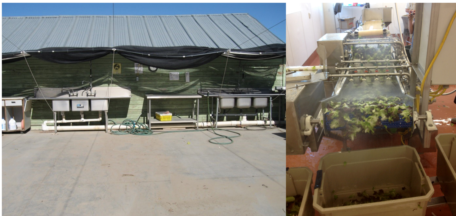
Figure 36. Multipurpose wash and rinse tubs on medium-scale farms (left), and a processing line designed especially for salad greens (right).
