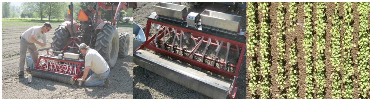
Figure 12. A 16-row mechanical seeder (left and center). Arugula (10 rows) mechanically seeded (right).
