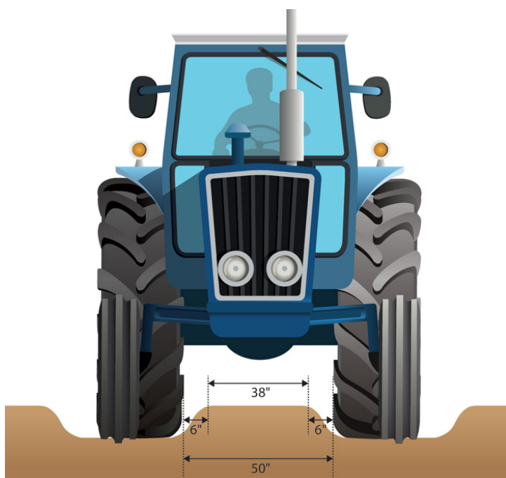
Figure 11. Base bed width on the inside space between the tires of your tractor. Subtract 12 inches and this will be the bed-planting surface. (Adapted with permission from Sahar Dabirian, WSU)
