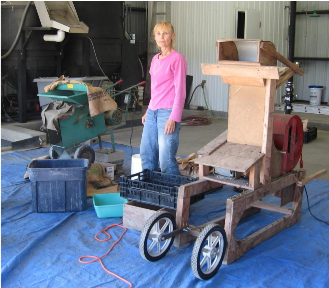
Figure 13. Small-scale thresher (left) and seed cleaner (right) used at WSU Mount Vernon NWREC.
