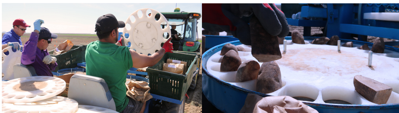
A simple switch of the discs between plots allows for spacing to go from 12 to 8 inches. Treatments included 8, 10, 12, 14, and 16 inches.
