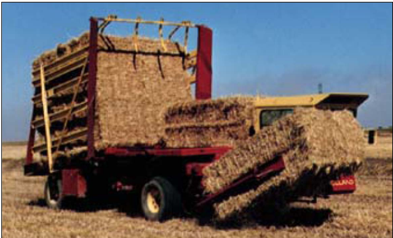
Figure 110: Road-siding Process (Large Bales: 1.2 × 1.2 × 2.4 m)
