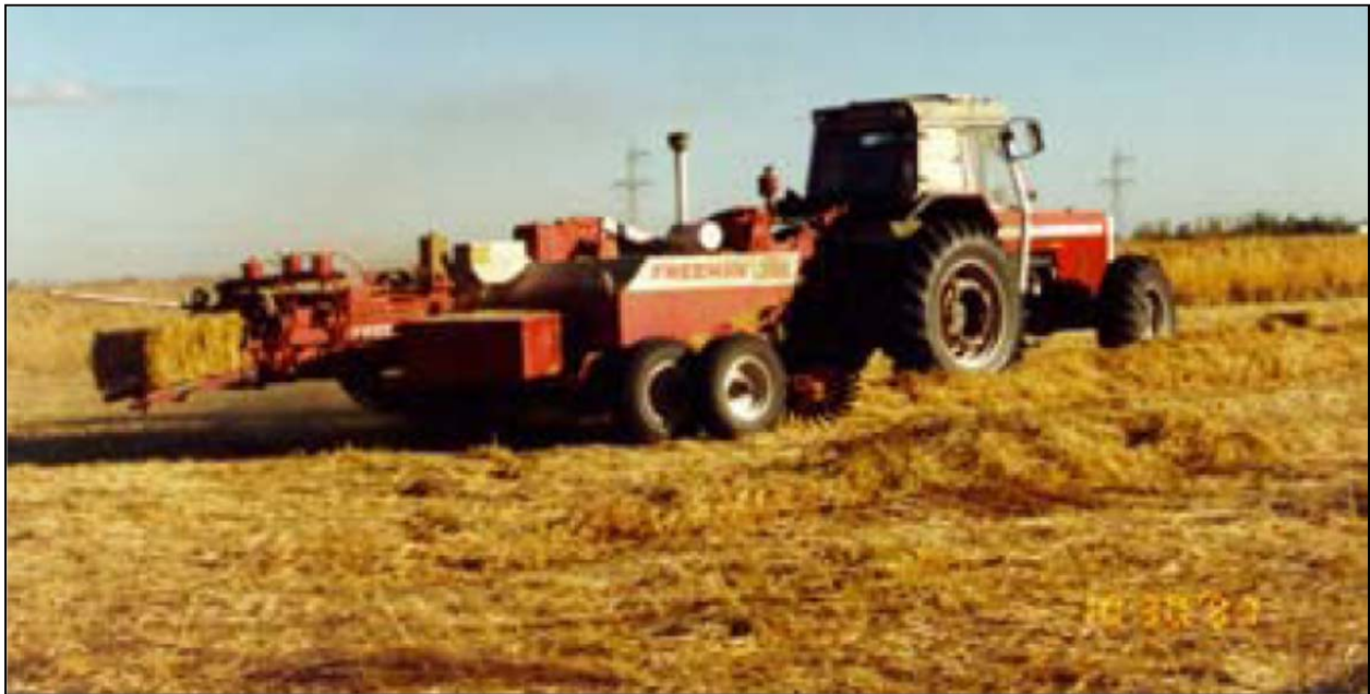
Figure 109: Baling Process (Small Bales: 0.4 x 0.6 x 1.2 m)
