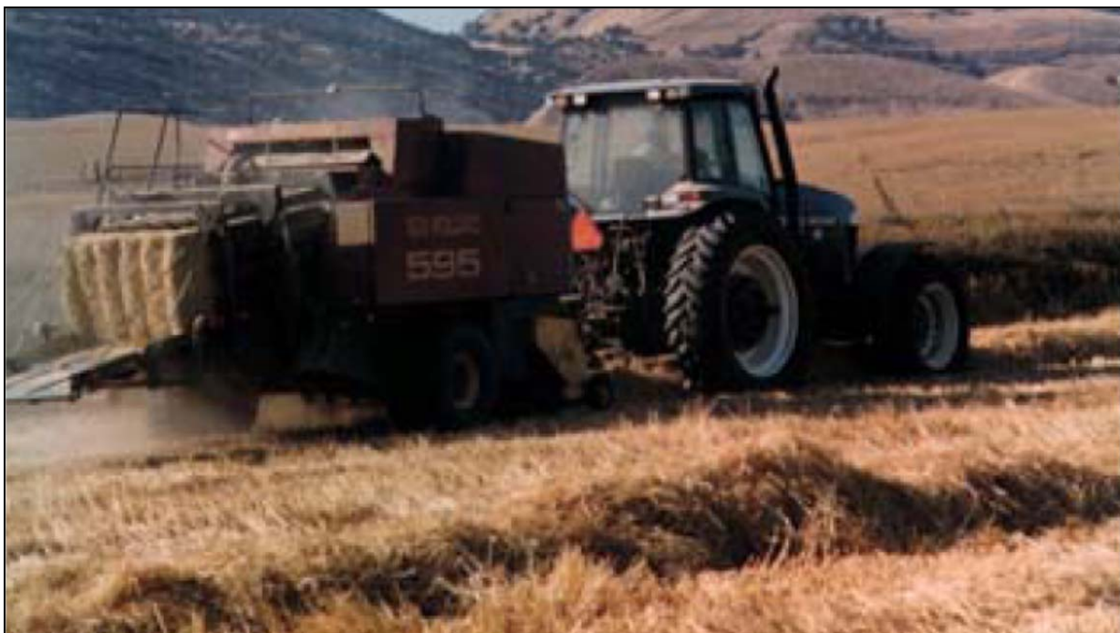
Figure 108: Baling Process (Large Bales: 1.2 × 1.2 × 2.4 m)
