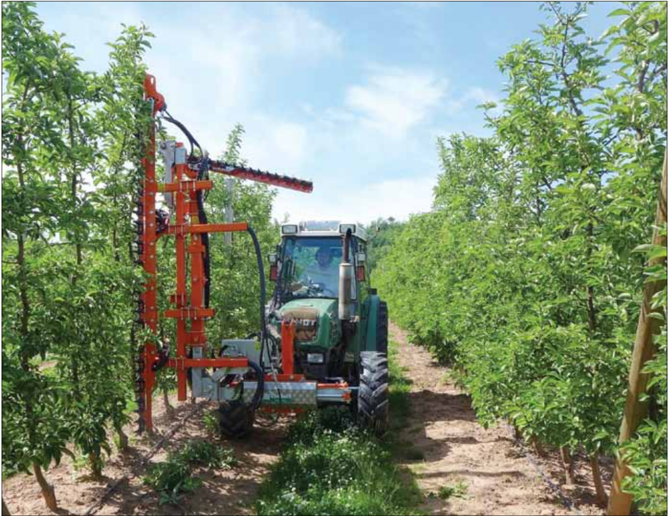
A tractor-mounted hedger at work in an orchard in Nova Scotia's Annapolis Valley. Keeping tree foliage tight to the trellis wire allows for more efficient tending and harvesting. (Perennia photos)
