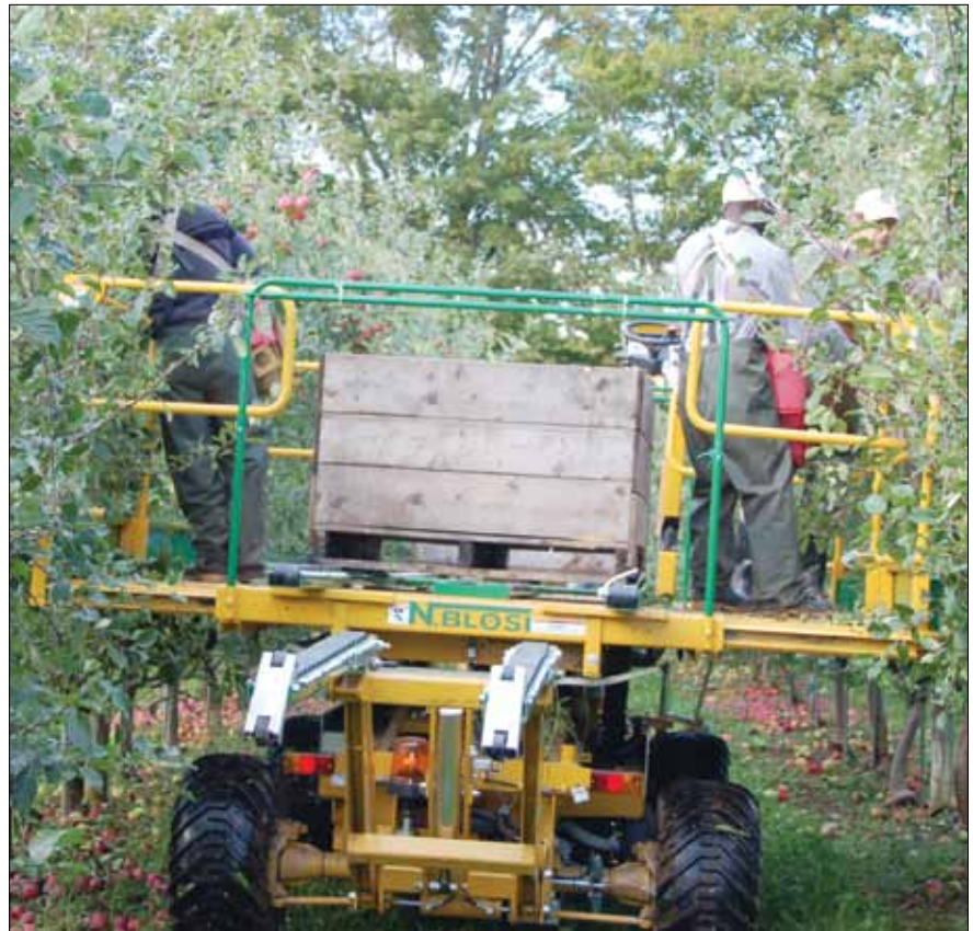
A mobile platform traversing the rows of trees, with workers and apple bin aboard – far less labour-intensive than climbing up and down ladders!
