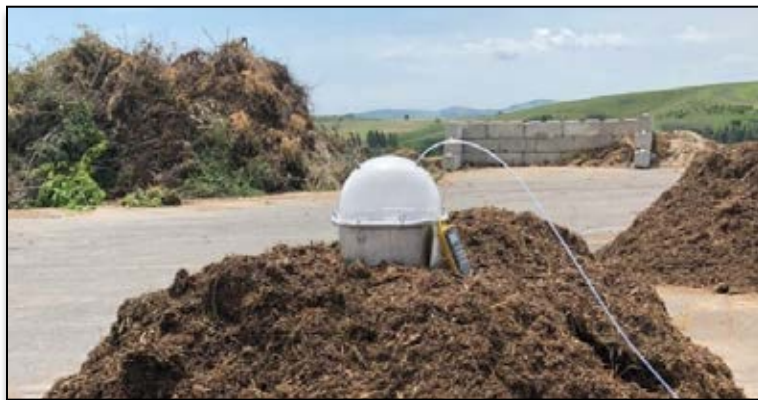
Figure 3: Photograph of flux isolation chamber at top of the 5% biochar pile B in row 2. View is looking to the southeast.
