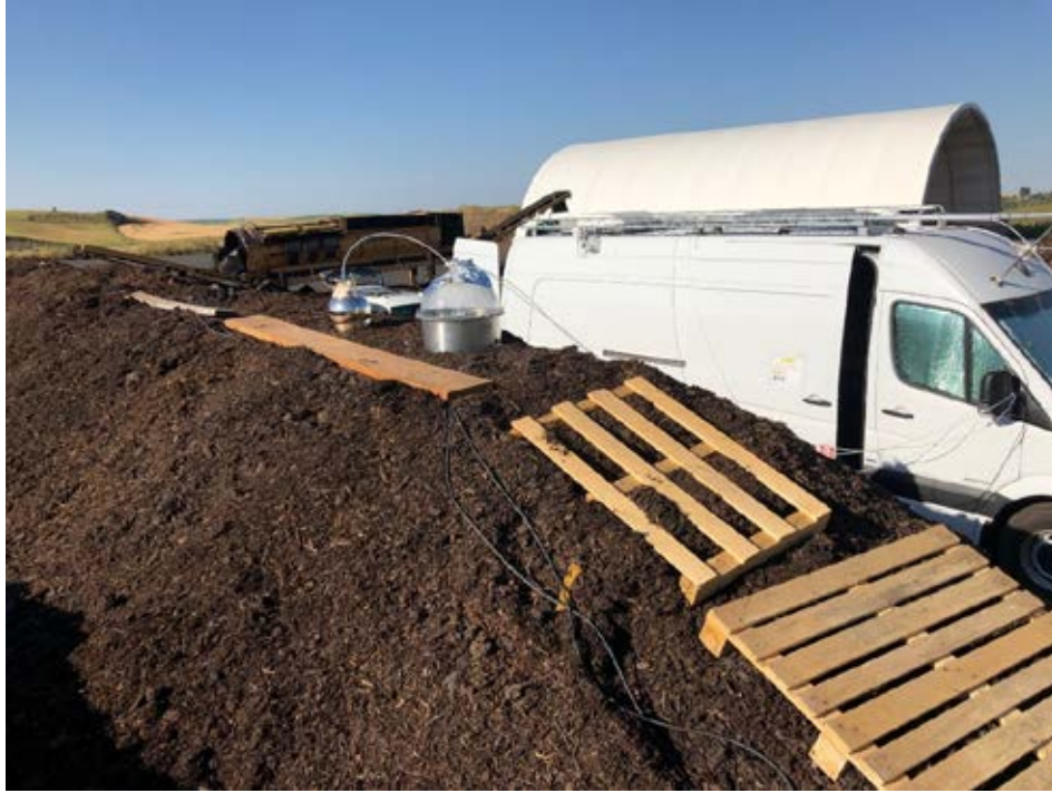
Figure 3: Surface flux isolation chamber at sampling location #1 with instrumented van in background.
