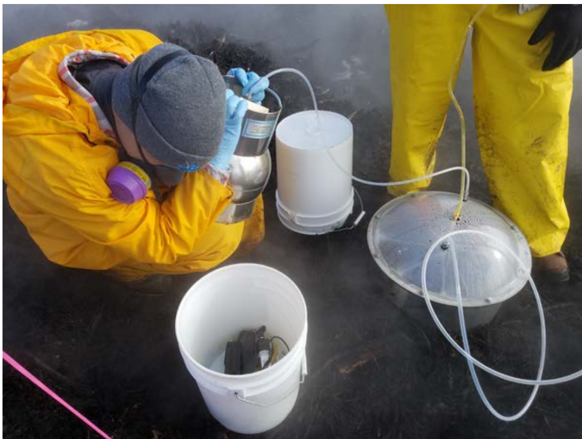
Figure 33: Surface flux sampling from a reversing aeration system conducted in March 2018 at Lenz Enterprises. The positive aeration condition is shown. Note water vapor vented from the pile is condensing in the colder ambient air and the heavy condensation in the surface flux isolation chamber where water is beading and running down the Plexiglas dome surface. (Photo: Doug Collins, WSU Puyallup)
