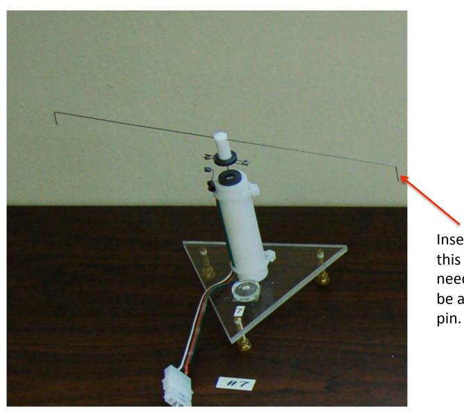
Insert insect pin into this bent hypodermic needle. There should be a hole to insert the pin.
