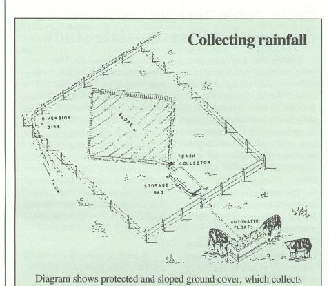
precipitation for storage bag. Float maintains proper water level in tank.
