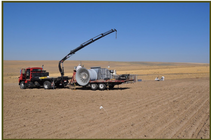
Figure 1. Portable wind tunnel used to collect windblown sediment from soils amended with biosolids at Lind, Washington. The photo was taken after sowing wheat in September 2015.
