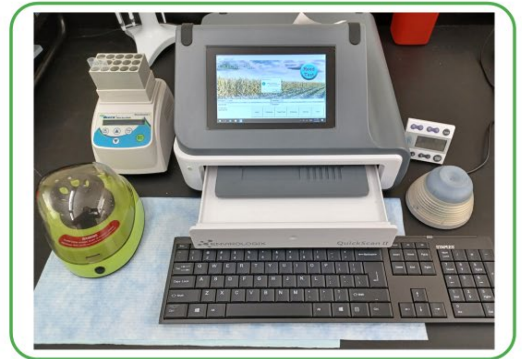
Proposed workstation with QuickScan system and EnviroLogix-provided accessories for Rapid FN test *Wheat mill/grinder not included
