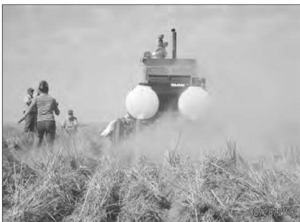
Fig. 1. WSU Lind drill with shovel-type openers on two ranks. This prototype has a 17-inch row spacing, solid packer wheels, and the frame is located high off the ground to allow clearance of high quantities of residue. We have had no plugging problems with this prototype in two years of testing.
