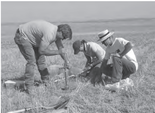
Fig. 1. Scientists and a research technician measure surface soil bulk density in a no-till fallow plot on the Mike Nichols farm in the western portion of the Horse Heaven Hills.
