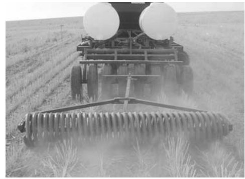
Fig. 1. An air drill is used to broadcast camelina seed on the soil surface followed by a coil packer to press the seed into the soil.
