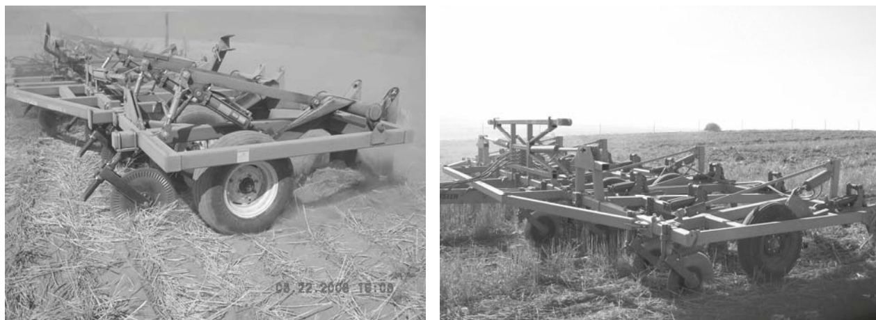
Fig. 1. The Great Plains (left) Duratech Haybuster (right) undercutters shown here slice below the soil surface with minimum surface soil lifting to completely sever capillary pores to halt liquid water movement towards the soil surface as required to retain seed-zone moisture in summer fallow in the low-precipitation region. All undercutters sold to farmers through the PNW Undercutter Project are rigged to deliver either aqua or anhydrous nitrogen during primary spring tillage.
